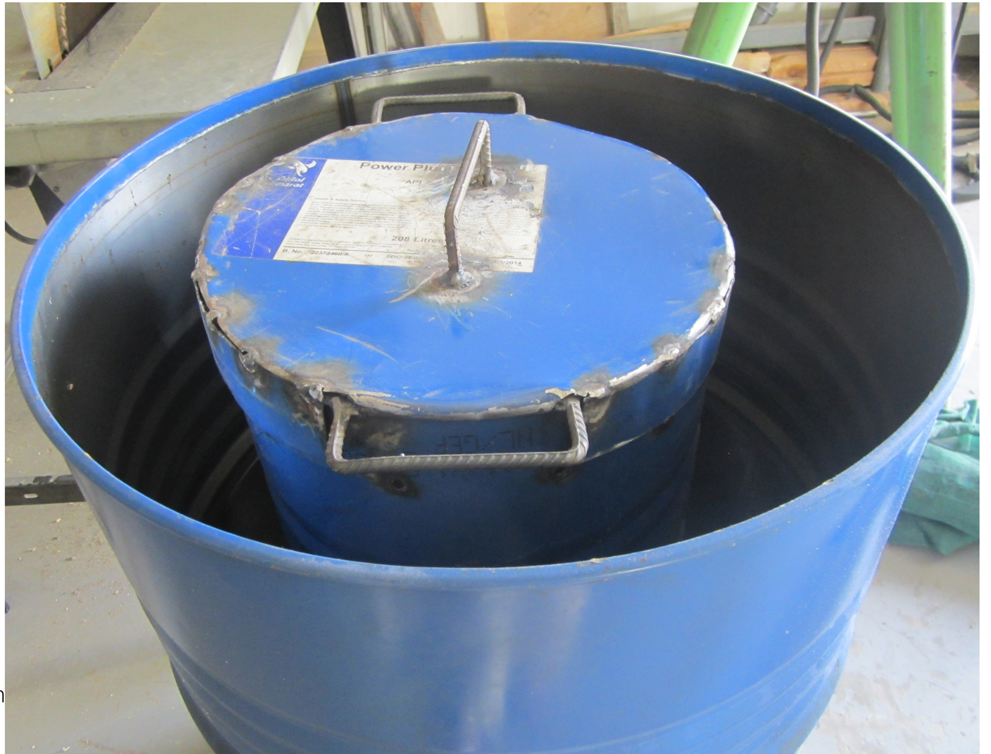
Figure 1: Setup of the pilot scale facility fabricated at ICBA to produce biochar
