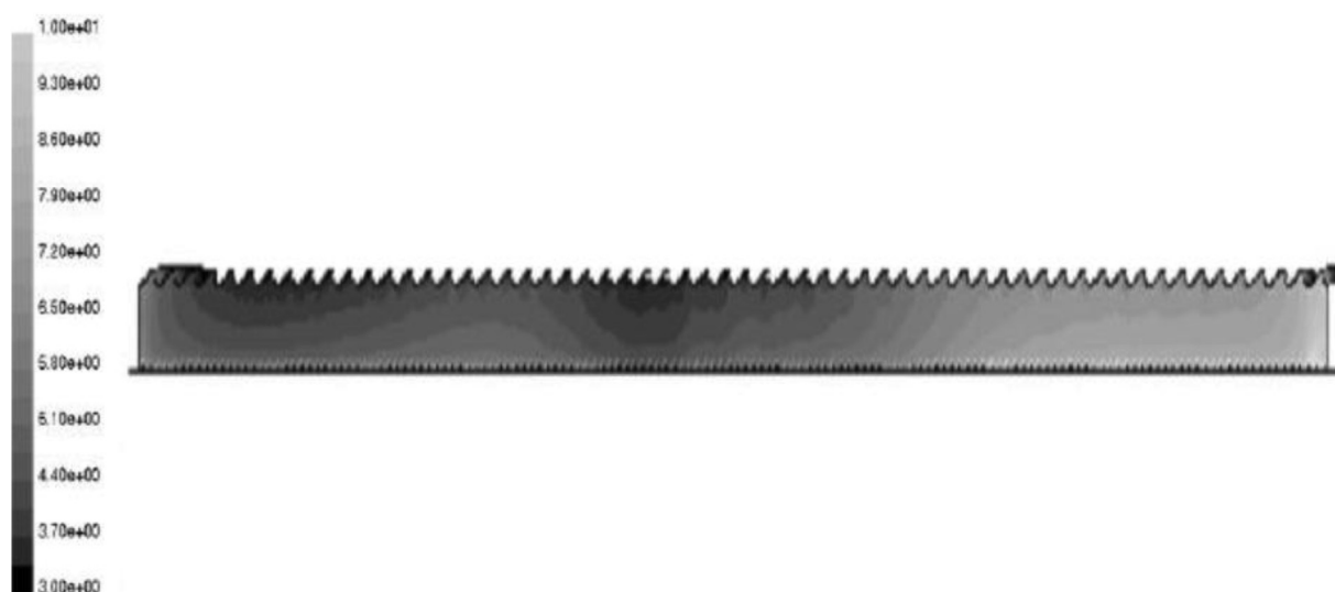
Fig. 10 – Carbon dioxide dispersion in a 60 span Venlo-type glasshouse with crops (after Reichrath and Davies 2001).
