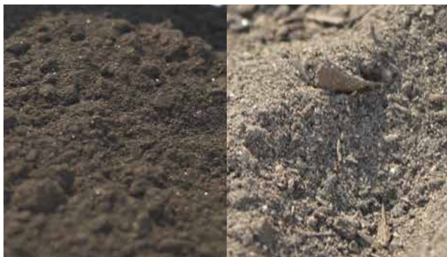
The color of biochar from conacarpus (left) is dark black and biochar from date palm (right) is grayish black
